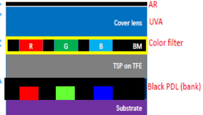
Pol-less, CF on TFE structure
