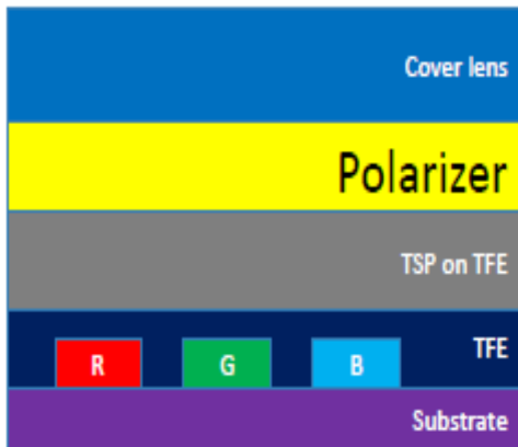
Common OLED stack-up structure
